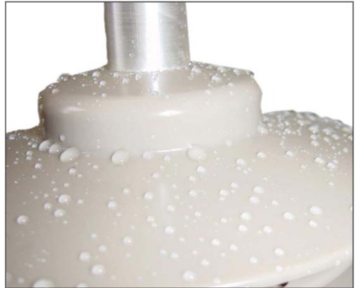
With hydrophobicity (HCEP) - HCEP does not become resistively conductive when exposed to moisture
